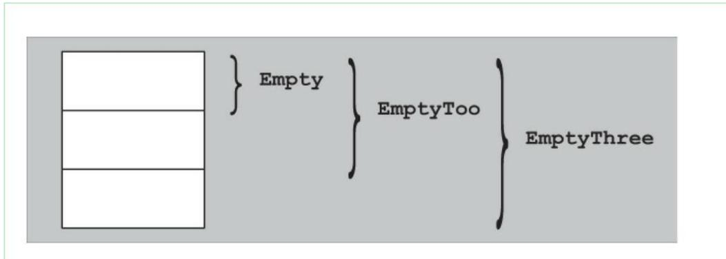
Figure 21.2. Layout of EmptyThree by a compiler that does not implement the EBCO
